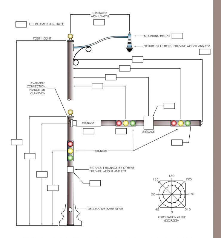
PLEASE FILL IN THE BOXES TO ENSURE THE MOST ACCURATE SPECIFICATIONS FOR YOUR PROJECT. THIS INCLUDES GAUGE AND DIAMETER OF POLE SHAFT, SIZE OF BASE, AND ANCHOR BOLT SIZE. PLEASE NOTE WEIGHT AND EPA VALUES FOR ALL MOUNTED FIXTURES.
